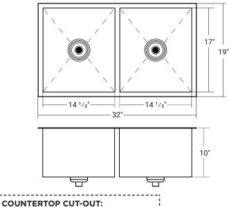
It is recommended that the hole for the sink be cut  $\mathcal{V}_2''$  x  $\mathcal{V}_2''$  smaller than the inside bowl dimensions.
