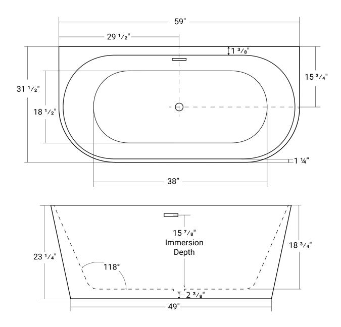
If the Semi-freestanding tub is going against any wall, the tub to be installed with the supplied tiling flange.
