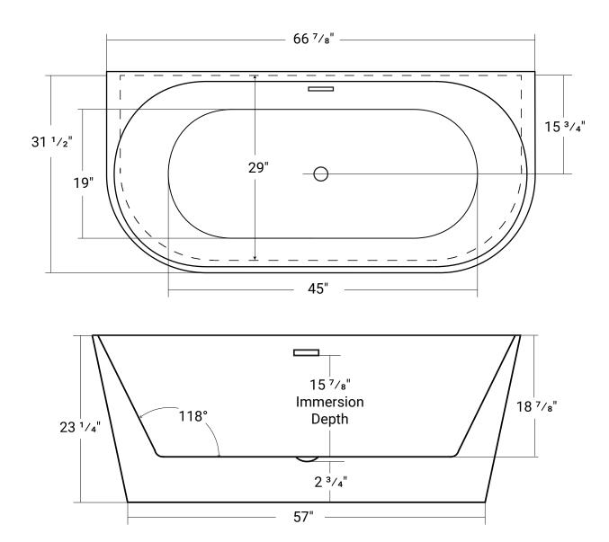
If the Semi-freestanding tub is going against any wall, the tub to be installed with the supplied tiling flange.
