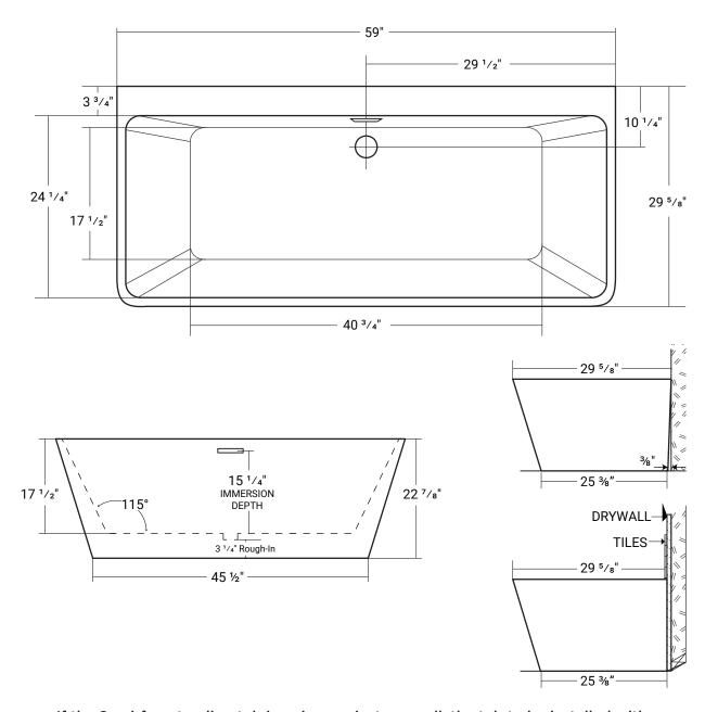
If the Semi-freestanding tub is going against any wall, the tub to be installed with the supplied tiling flange.
