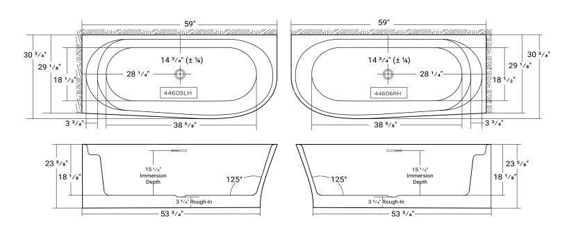
If the Semi-freestanding tub is going against any wall, the tub to be installed with the supplied tiling flange.
