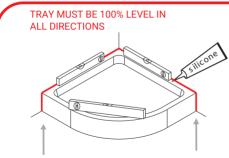
Ensure the shower tray is level in all directions and is properly sealed to the wall. The wall must be tiled down to the top edge of the tray. Do not angle out the bottom tile.
